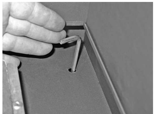
- Adjust height with Allenkey no. 5.
