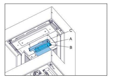
The appliance is factory supplied with a baffle plate. This baffle plate is located at the top of the combustion chamber, just before the connection with the concentric flue. The baffle plate only remains on location, if a restriction plate needs to be mounted. Refer 4.2.9.
