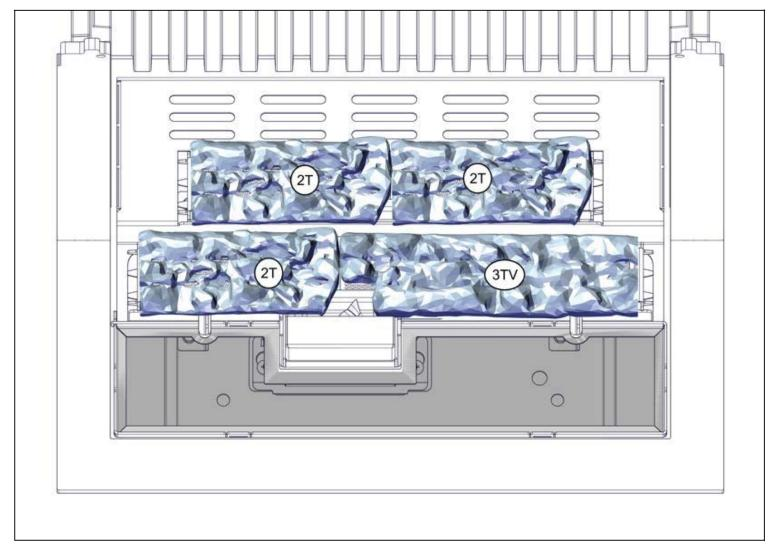
2. Put the ceramic ember grates on the lower and upper main burner, as shown below. Refer to *2.6* for the numbers of the items.
