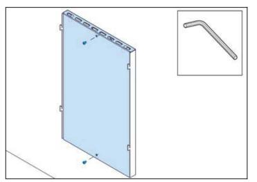
5. Put the appliance on the support frame. Make sure that all four hooks of the support frame go into the slots on the back of the appliance. Lower the appliance until it hangs tightly on the support frame.
