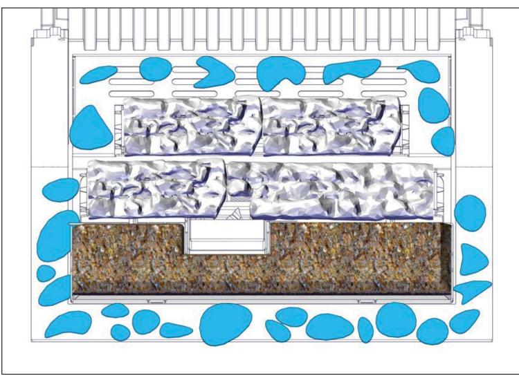
5. Put the charcoal pieces and chips of wood at the designated places around the burner bed. Refer to *2.6* for the numbers of the items.
