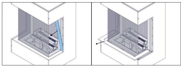
3. Unlock the fastening levers on the top left and right of the glass panes.
