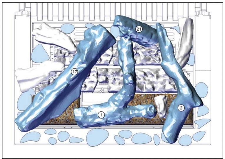
6. Put the logs on the burner bed. Refer to 2.6 for the numbers of the items.
