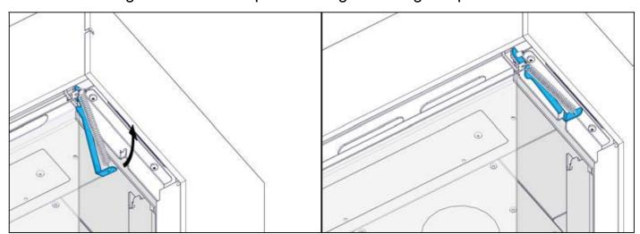
6. Install the front panel and side panels.
