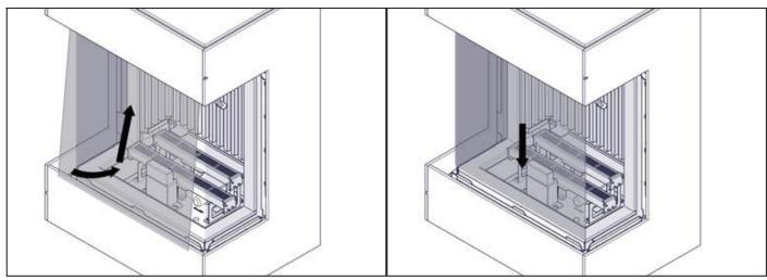
5. Lock the fastening levers on the top left and right of the glass panes.
