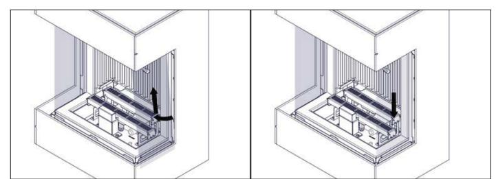
3. Tighten the screws left and right of the top side strips.4.
